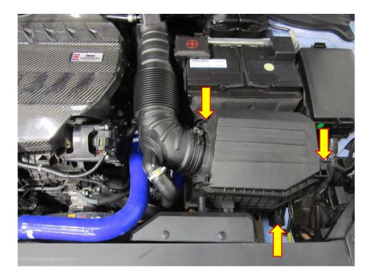
2. Next you need to remove the two fasteners that hold the air scoop to the front of the airbox. To do this simply push the pin in the centre of the fastener inwards, then prise up the fastener with a flat blade screwdriver/trim removal tool.
