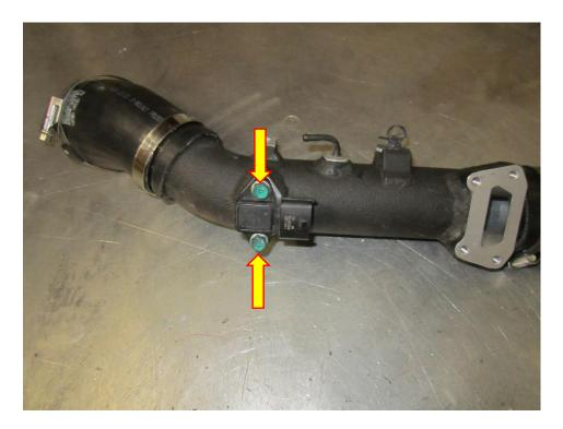
**11.** Take the FMBP4 hard pipe and attach the two silicon hoses as shown in the picture below. Do not tighten the hose clamps up as you may need to adjust the positioning of the hoses. Fit the map sensor using the OE M6 fasteners.
